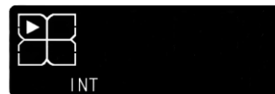
When powered up, pump will return to its previous status before power-off
